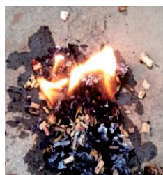
Oiled chips produced by mixing waste cooking oil and sorghum chips (left) Burning oiled chips (right)
